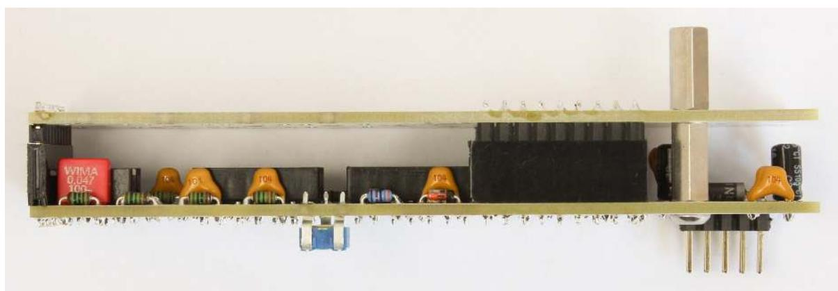
Disconnect the boards. Don't forget to place the **ICs** into the sockets (2x **TL074**, 1x **V2164D**, 1x **LF398**). There is a notch on each IC that has to match with the notch on the socket.
