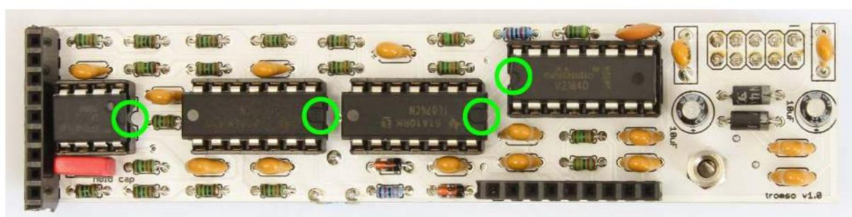
Great, you are done now with the bottom board! Before moving to the next one make the last check that all parts are on the right place and every joint is properly soldered.
