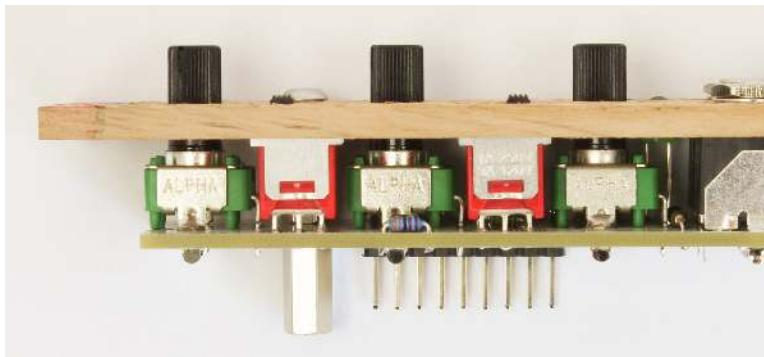
Then turn the unit facing with PCB upwards. Make sure that everything is properly aligned. Push the **switches** and **LED** to be sure that they come through the panel. Now you are finally ready to solder all these inserted parts.
