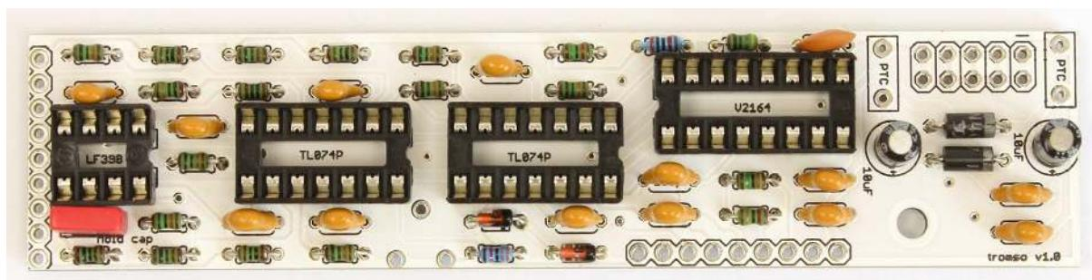
Turn around the PCB to solder the **2x5 pin male header** and solder it. Be careful to solder the headers straight. You may first solder one of the pin, take the board in your hand and re-heat that pin while you are adjusting the header straight. Add also the **trimmer**.
