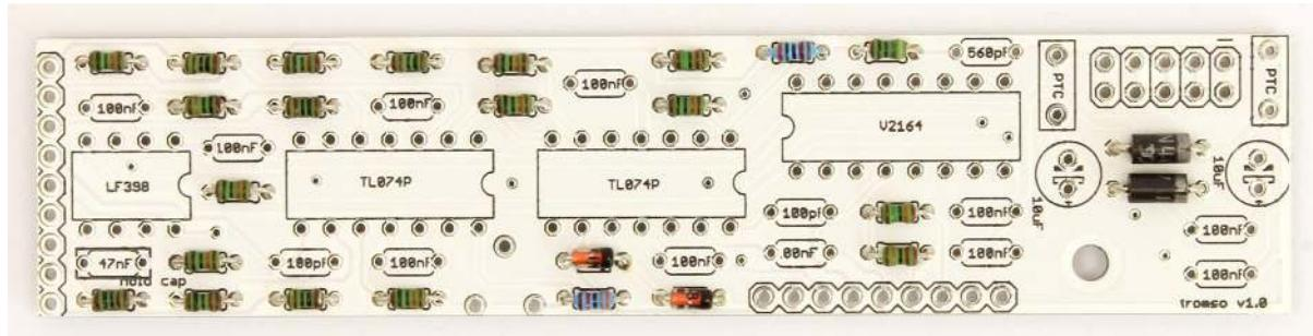
Now you can move to soldering the **IC sockets** (be aware of the right direction, there is a notch on the sockets that has to match with the sign on PCB):
