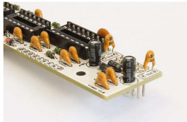
To finish soldering of the bottom board you have to connect the female headers with the male headers from the Top board bag. Use your flush cutters to get two pieces of **1x9 female pinheaders** (you will always lose one pin when cutting the female headers, so be sure to cut it always after the last required pin).
