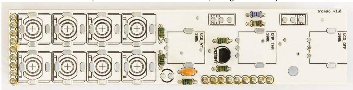
Insert now all the other parts (**jack connectors, potentiometers, switches and LED**) but do not solder them yet:
