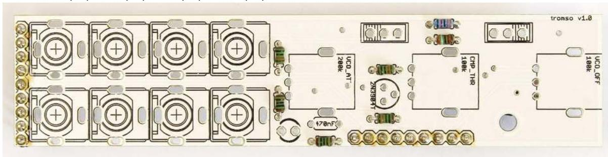
Then insert and solder some other parts (**capacitor and transistor**):
