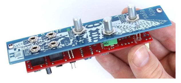
Check the position of all the parts if they are flat on the board, push the LEDs to the panel and do the soldering.
