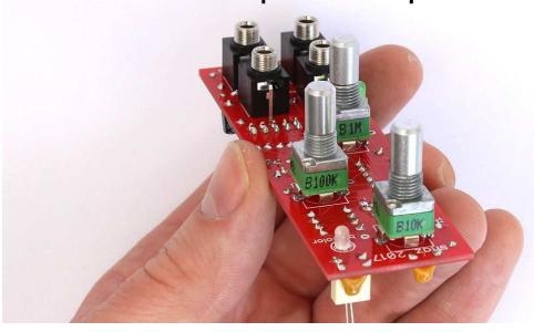
Place the **front panel** on and mount the pots with **nuts**.
