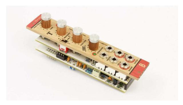
Before you connect anything, make sure that your system is disconnected from power. Also double check the polarity of the ribbon cable, the red cable should match the -12V rail both on the module and on the bus board!
