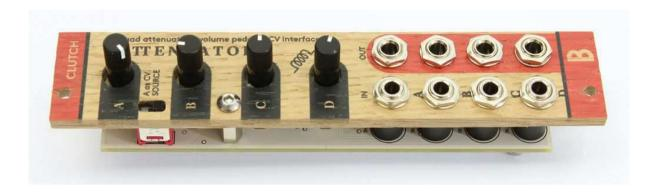
Check that all all the components came through easily (especially the switch). Finally you are ready to solder rest of the components.
