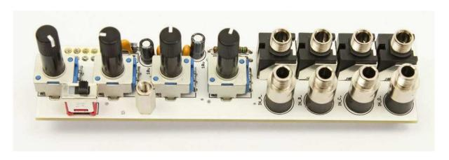
Lay down the **front panel** on the board and add one **screw**, eight **washers** and eight **nuts**. (don't tighten the jack nuts too much as you may damage the panel!).
