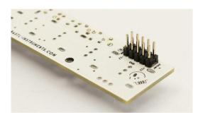
Turn around the PCB and solder **2x5 pin male pinheader**. Be careful to solder it straight. You may first solder one of the pin, then take the board in your hand and re-heat that pin while pressing down on the header to align it (be careful though, you don't want to touch the pin you are heating up). Wait for it to cool and solder the rest of the pins.
