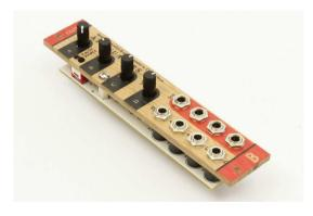
Congratulations! You have made it through. Before you connect anything, make sure that your system is disconnected from power. Also double check the polarity of the ribbon cable, the red cable should match the -12V rail both on the module and on the bus board!
