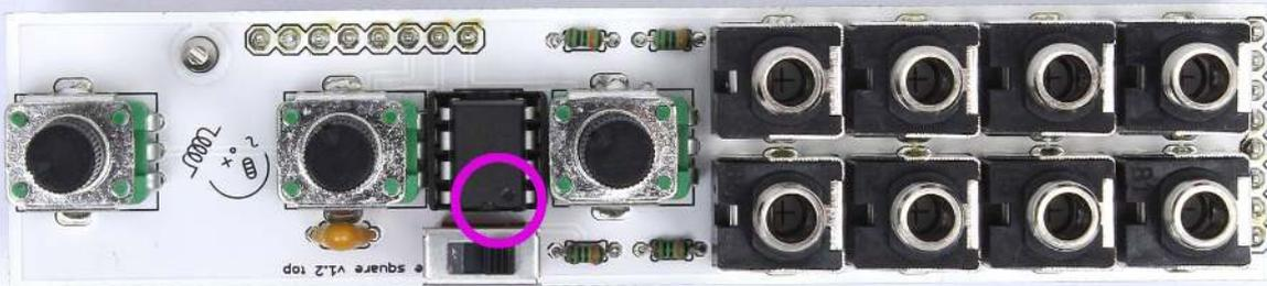
Congratulations! You have made it through. Now just connect the boards, add the knobs and your NOISE SQUARE is ready to go! Before you connect anything, make sure that your system is disconnected from power. Also double check the polarity of the ribbon cable, the red cable should match the -12V rail both on the module and on the bus board!
