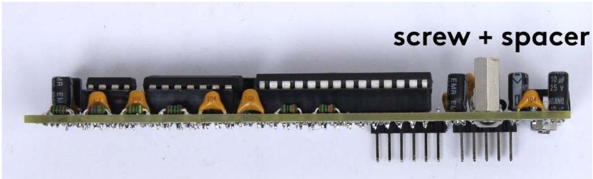
You need **two 1x8 male pinheaders** now. Cut them with your flush cutters. Place the **female headers** on the bottom board with the male pins inserted. Connect the boards together and mount them with the other spacer. Now you can **solder the headers** on both boards.
